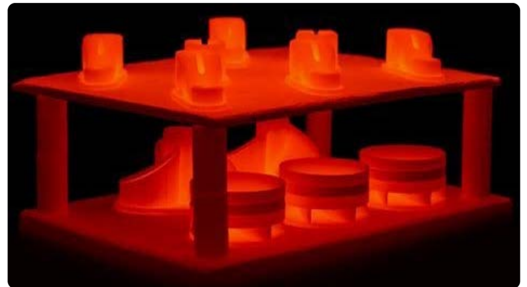
Parts in a sintering furnace
